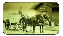
**This** is a Contractors Suspension Body Dumping following illustrations in the May, 1906, Carriage Monthly. To increase capacity, slanting boards were added as shown
